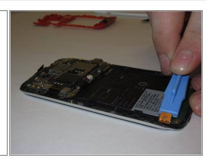
• Remove the connector on left side of the Navigation board by unplugging/prying the orange ribbon.
