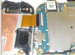
Remove the gold ribbon cable by lifting tab at the back of the socket, using a spudger or tweezers.
