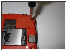
Use a Torx T5 screwdriver to unscrew and remove five 3.0 mm screws from the rear frame.
