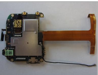
Gently pull the logic board to the right and it will disconnect from the chassis.
