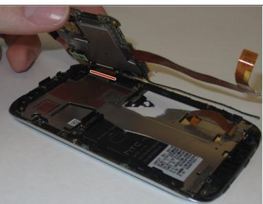
• Gently pry logic board from the casing by lifting the left side up, as if there was a hinge on the right, folding it over the right edge where you will see a gold/orange ribbon cable.
