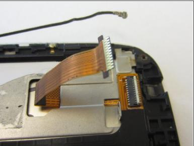
Disconnect gold ribbon cable connecting screen to logic board by pulling cable out gently.
