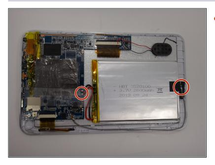
Locate the batteries' connection points.
