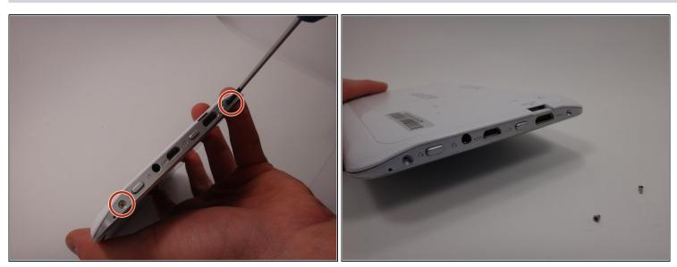
Use a Phillips #00 screwdriver to remove the two 4mm screws found on the top edge of the tablet near the power button.
