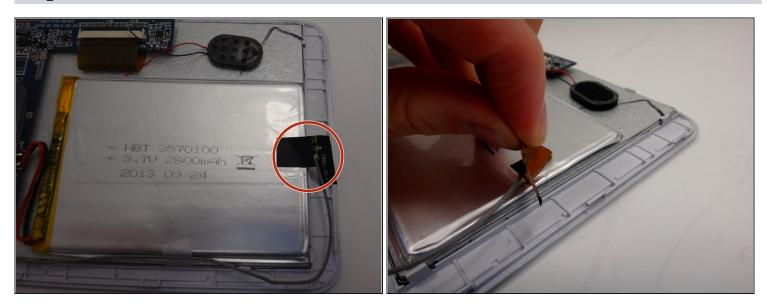
Peel the black sticker off the battery to disconnect the wifi antennae.
