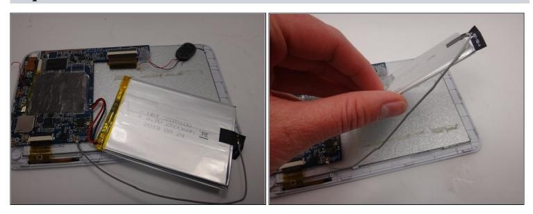
• Remove the old battery and replace it with the new battery.
