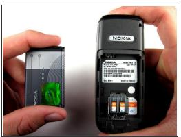
• Use a plastic opening tool (or your finger) to gently pry the battery out of the battery slot on the back of the phone.
