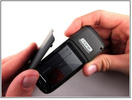
Place your thumb on the middle of the back cover and push it toward the bottom of the phone to slide the cover off.
