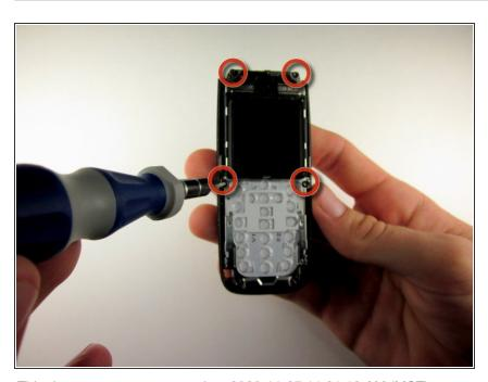
Remove the 4 screws surrounding the screen using the precision T6 screwdriver.
