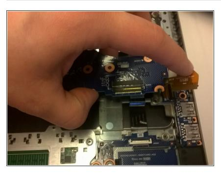
If there is any resistance you should double-check that all cables and screws have been removed or disconnected.
