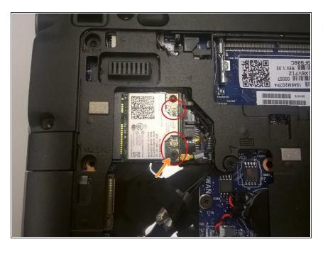
The two red circles indicate where antennas plugged in. They simply pop upwards.
