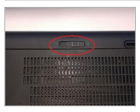
The bottom cover will then slide towards the bottom of the picture, and can be removed.
