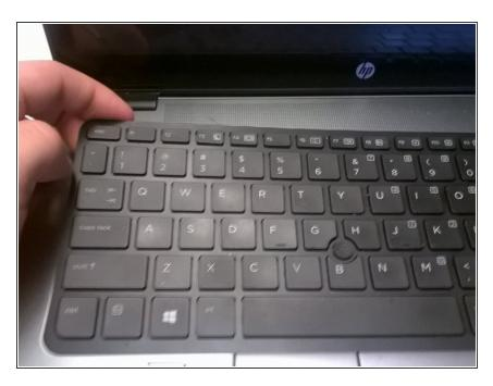
You should pull the top edge loose, and slide the keyboard upward.
