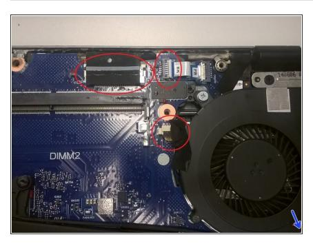
The fan is also held by a screw in the bottom right. This was partially cut off in the image.
