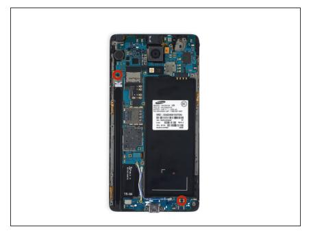
Remove the two 2.9 mm Phillips #00 screws.
