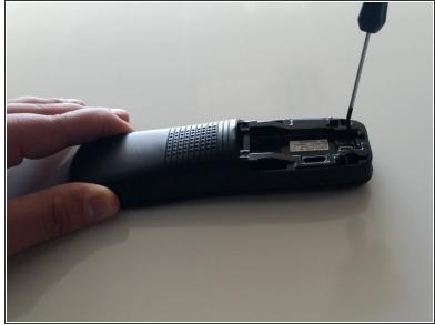
Remove the two 9mm Phillips #1 screws in the battery compartment.
