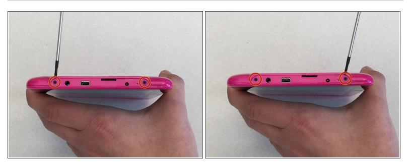
Remove the two 8mm Phillips Head screws located at the bottom of your device.
