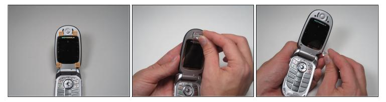
• Remove the four rubber stoppers from around the screen with a pin to reveal four screws.
