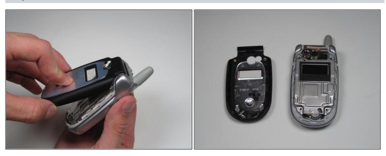
• With the edges separated, close the phone and lift off the faceplate with your fingers.
