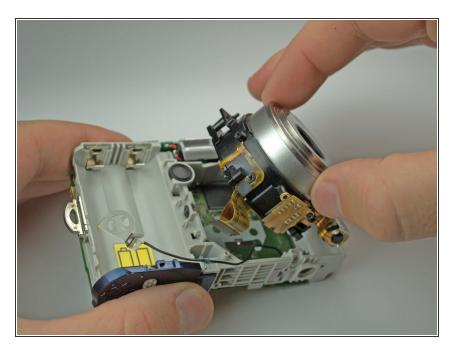
There is a screw behind flash tube holding lens. Remove it, then gently pull the lens out. Be sure that the lens's ribbon clears the motherboard.
