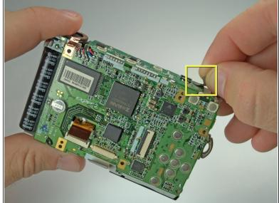
Remove the tape on the top of the logic board.
