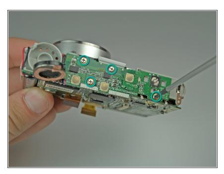
Remove the 4 Phillips #00 screws holding the top of the logic board onto the camera frame.
