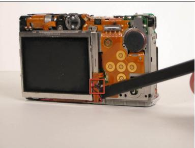
Use the flat end of the spudger to lift up the small black connector from the back side of the motherboard. The connector should just lift straight up.
