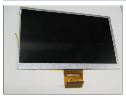
This is the component once it is removed from the screen casing.
