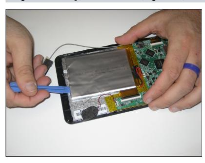
Remove the battery by first removing the electrical tape holding it down. Then begin gently prying underneath it and around the edges with your plastic opening tool, until the battery is loose.
