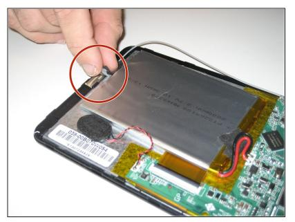
Remove the antenna by peeling back the tape holding the antenna to the casing.
