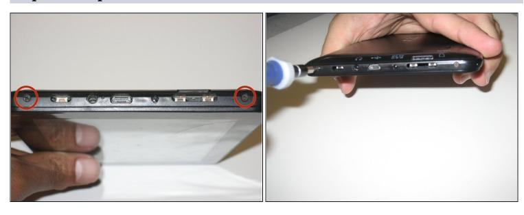
• Remove the two 2.5mm Phillips head screws before attempting to remove the screen from the device.
