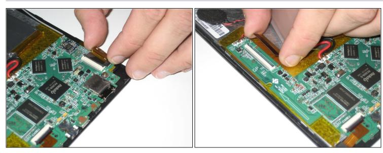
• Unclip the ribbon cables from the motherboard by lifting up on their latches (the black portions that the cables feed into) and gently pulling the cables.
