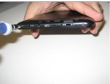
Remove the two 2.5mm Phillips head screws before attempting to remove the screen from the device.
