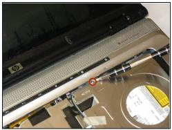
Remove the four 5.8 mm Phillips screws securing the top cover to the lower case.
