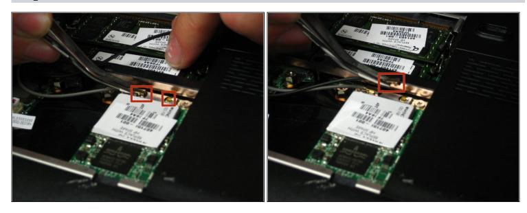
• Use a pair of <u>tweezers</u> to disconnect both antennas from their sockets on the wireless card. These are snap-on connectors, so simply pull them straight up to snap them off the studs on the card.
