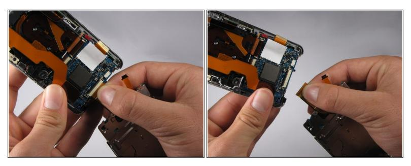
Disconnect the large ribbon-wire by pulling on the large ribbon-wire where it connects to the motherboard.
