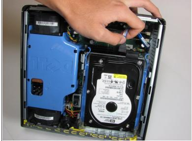
Unplug the blue cable that connects the hard drive to the motherboard.
