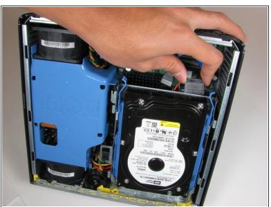
Unplug the power supply, distinguished by its red and yellow wires (yellow wire obscured from view).
