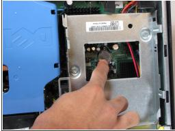
Upon replacement, simply push the battery into the motherboard.
