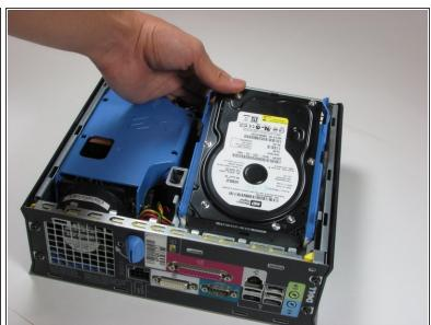
Slide the Hard Drive out while squeezing the tabs.
