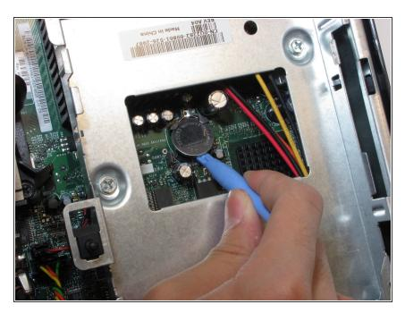
Lift the battery out of the motherboard.
