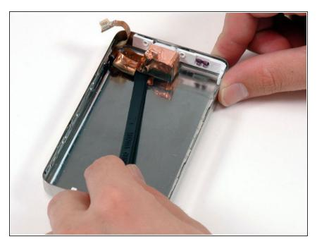
Slide a spudger beneath the orange headphone jack cable and use it to pry the cable up from the rear panel.
