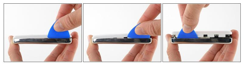
Insert an opening pick as far as possible into the seam between the plastic front and the metal rear panel, on the right edge of the iPod.
