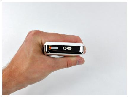
Before opening your iPod, ensure that the hold switch is in the locked position. The orange bar should be visible, indicating hold is active.
