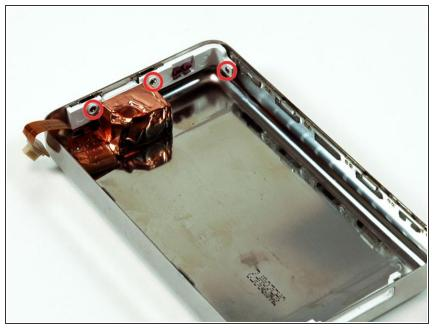
Remove the 3 silver Philips screws securing the headphone jack to the rear panel.
