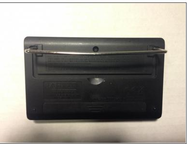
First, open the metal stand to access the screws without damaging the body.
