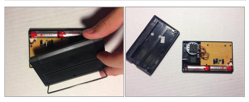
Remove the back casing to reveal the inner circuitry.
