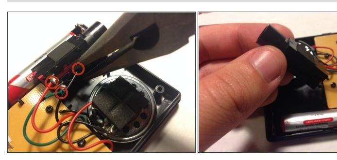
Snip the wires attached to the input jack port using the wire cutter as close to the input jack port as possible.
