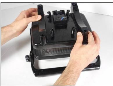
Lift the plastic lower heating element up and place to the side for reassembly. You have now disconnected the plug wiring completely.
