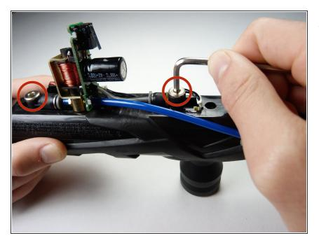
Remove the two 1-1/4" screws on either side of the circuit board using a 3/32" allen wrench.
