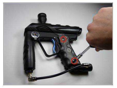
Remove the four 8mm screws on each side of the gun's grip using a Phillips #2 screwdriver.
