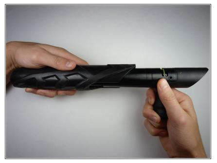
• Slide the metal body out of the plastic shell by holding one in each hand and gently pulling apart.
