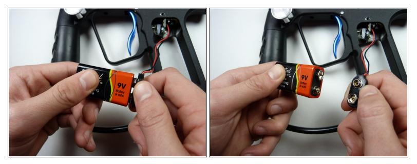
• Remove the 9V battery by unsnapping it.
