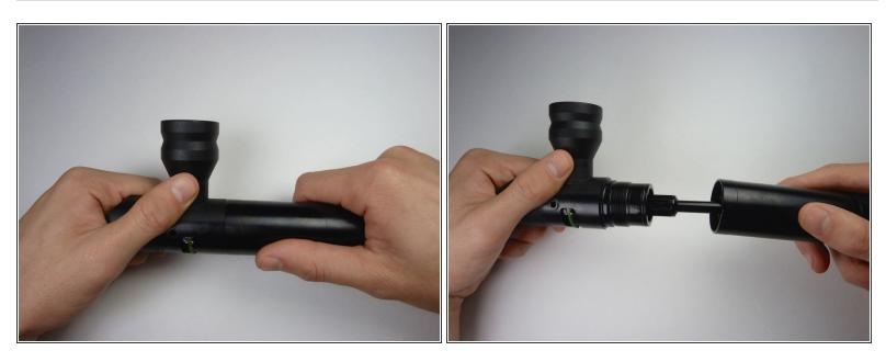
• Separate the front body breach from the fire chamber by rotating the breach counterclockwise.
