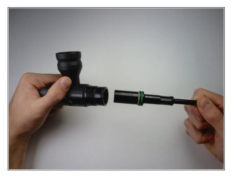
• Remove the bolt from the front body breach by gently pulling on the bolt.
