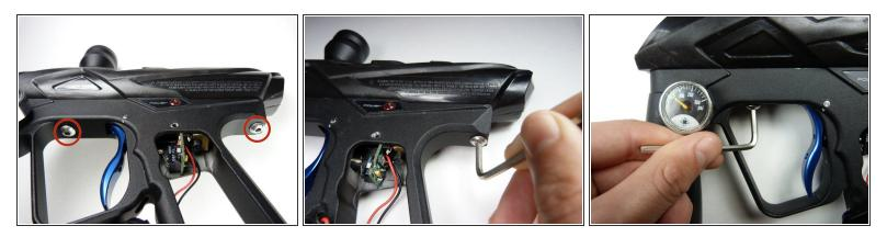
• Remove the front and rear 1" screws on the gun's grip frame using a 3/32" Allen Wrench.
