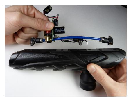
• Separate the solenoid from the gun's body by gently pulling it upwards.
