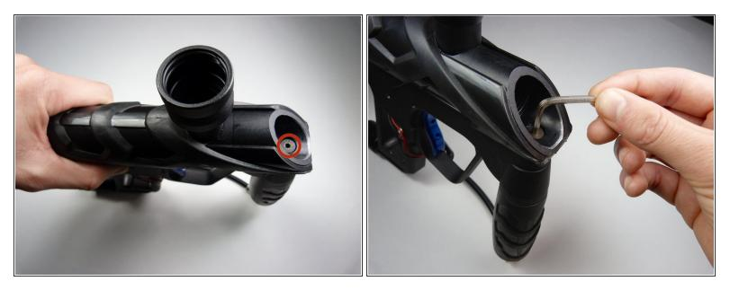
• Remove the 12 mm screw on the top of the grip frame using a 3/32" Allen wrench.
