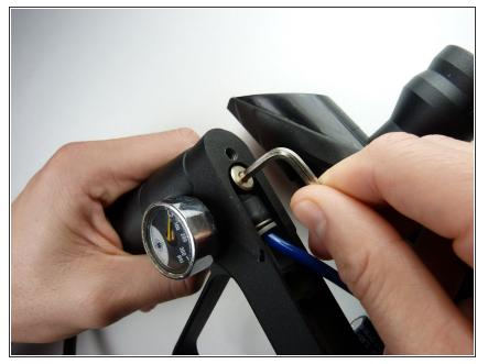
Remove the 1-1/4" screw that's attached to the blue tube above the front grip using a 3/32" Allen Wrench.
