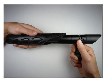
Slide the metal body out of the plastic shell by holding one in each hand and gently pulling apart.
