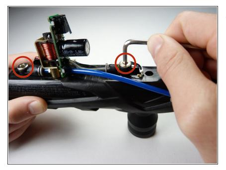
Remove the two 1-1/4" screws on either side of the circuit board using a 3/32" allen wrench.
