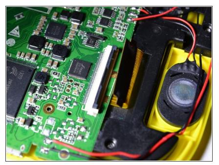
• Pull the two ribbon cables out so that they are no longer connected to the logic board.
