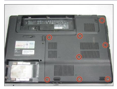
Remove the 8 screws from the back cover using the Phillips #00 screwdriver.
