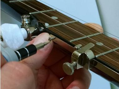
Use the flat head screw driver to insert and tighten the screws.
