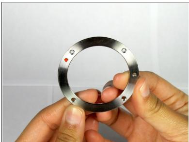
Remove the metal ring using the plastic opening tool.
