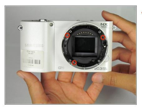
Remove the three 4.5 mm Phillips #000 head screws located inside the cover with a Phillips #000 screwdriver.
