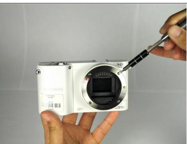
Unscrew the four 5.5 mm #000 Philips screws that are on the metal ring with a Philips #000 screwdriver.
