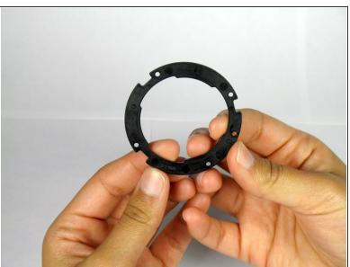
Remove the black plastic ring using the plastic opening tool.
