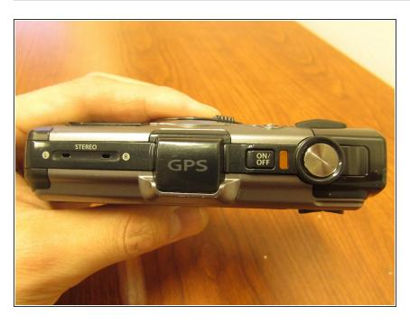
The top of the camera does not contain screws. You do not need to remove anything from the top of the camera.
