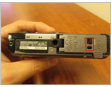
Release both latches on the battery compartment on the bottom of the camera to open the door.
