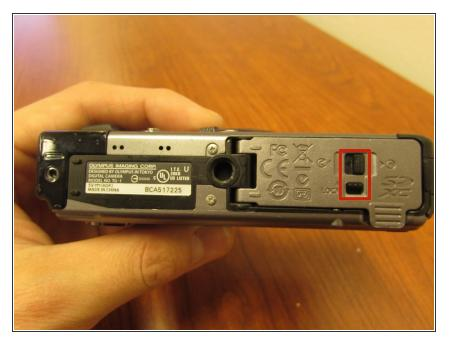
Release both latches on the battery compartment on the bottom of the camera to open the door.
