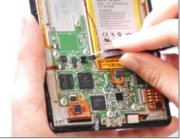
• Use <u>tweezers</u> to pinch in the sides of the vibrator cable and slide it out of its housing.
