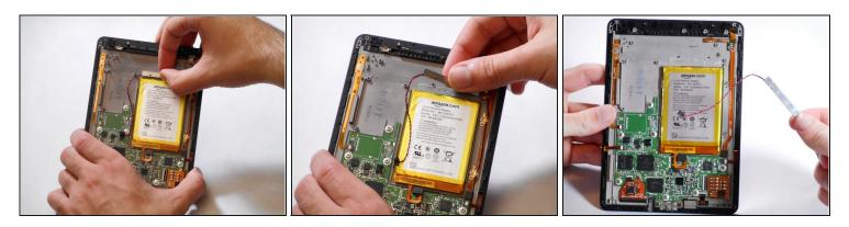
• Gently peel the vibrator off of the device.
