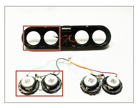
Each speaker is held down by two clips. On the front face of the speaker, push the speaker outward while pushing one of the clips that holds it down to the side. Repeat this on the other speaker and clip. The speakers should pop out. To reassemble your device, follow these instructions in reverse order.
