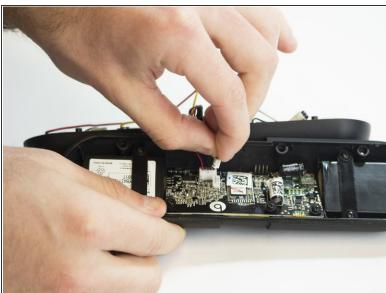
Carefully remove the black and red NFC sensor wires.
