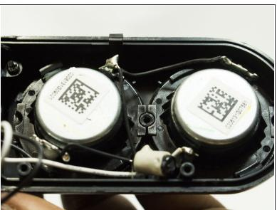
Using the Phillips #0 screwdriver, unscrew the two screws that holds the speakers down.
