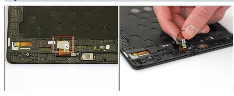
• Use a spudger or your fingers to remove the LCD connector from the display assembly.
