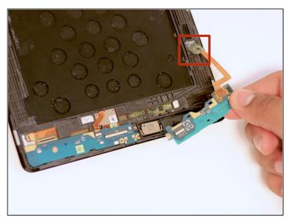
The daughterboard has an orange ribbon cable that is adhered to the device. Gently pull the ribbon up and remove the daughtboard.
