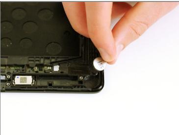
• Use a pair of <u>tweezers</u> to remove the vibrator from the device.
