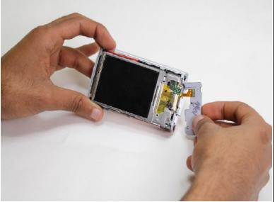
Using the screw driver, unscrew the one screw on the control panel board.
