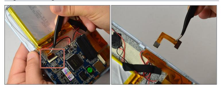
• Using a pair of <u>tweezers</u>, gently grasp the flex cable and pull it out while using your other hand to keep the camera in place. Once removed, your camera is now free and ready for replacement!
