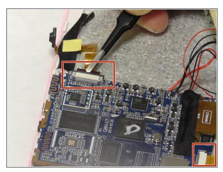
Using the small needle nose pliers, carefully remove the small yellow ribbons that are attached to the motherboard.
