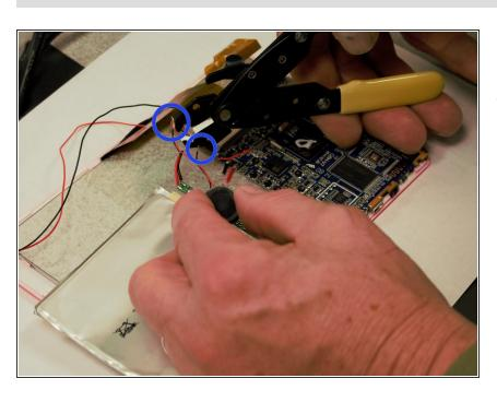
Strip both the red and black wires in the middle with a wire stripper/cutter tool. Do this for all wires that were cut, as well as for the wires on your new motherboard.
