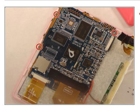
Remove all three screws holding down the motherboard, using the Phillips #00 Precision Screwdriver and slot in the Phillips Head PH #0.
