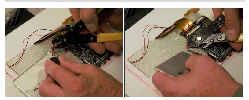
Cut the red and black wires that connect the battery, screen, camera, and speakers to the motherboard.
