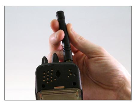
Twist the antenna counter-clockwise to unscrew it from the antenna jack.
