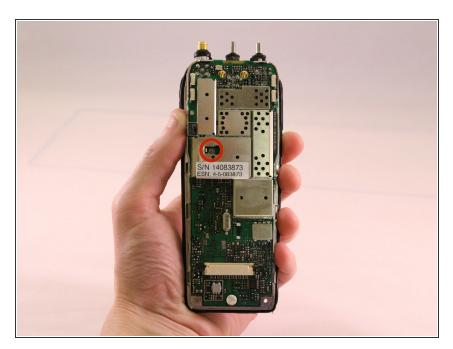
Using a T15 Torx screwdriver, unscrew the 3.8mm screw from the case.
