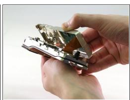
Using the plastic opening tool, pry the case apart.
