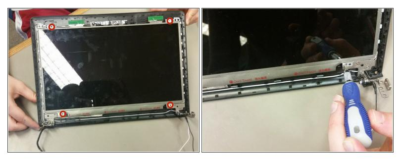
Unscrew the four M2.5x4mm Phillips screws. One screw is located at each corner.
