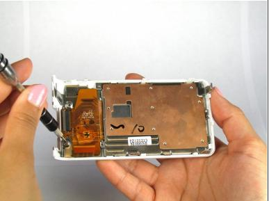
Remove all five 3mm Philips #000 screws from the inside of the back panel using the Philips #000 Screwdriver.
