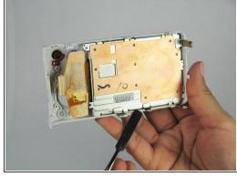
Use a metal tool to pick on the sides of the metal plate to remove the plate from the plastic tabs.
