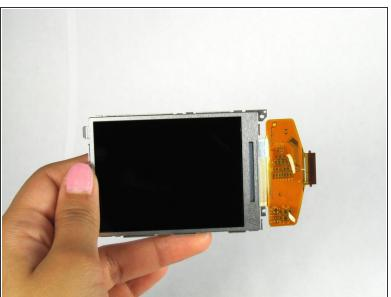
Separate the LCD from the back panel.
