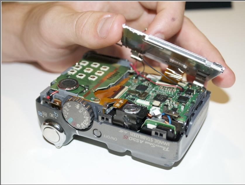
**⚠ CAUTION:** The LCD is connected to the motherboard with different wires and a ribbon. Using too much force may disconnect these parts.
