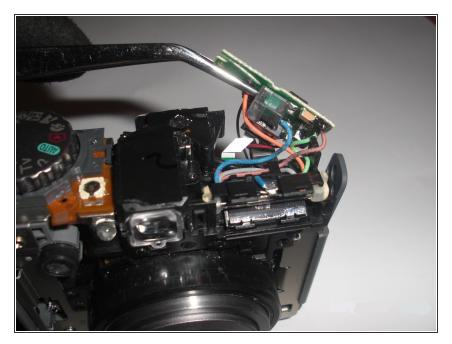
• Unsolder the cables under the circuit board.
