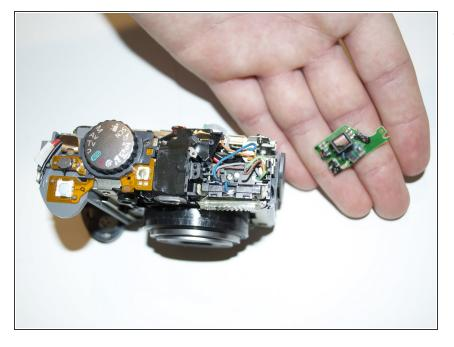
The flash logic board can now be removed from the camera and replaced.
