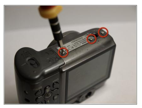
Remove the three screws located at the bottom of the camera using a Phillips #00 screwdriver.
