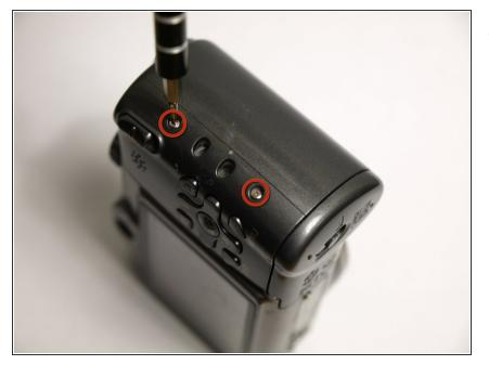
Remove the two screws located on the other side of the camera using a Phillips #00 screwdriver.
