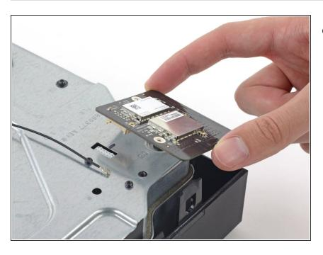
Lift straight up on the W-Fi board to disconnect it from its connector and remove it from the Xbox.
