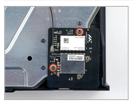
Remove the two 9.5 mm T9 Torx screws from the WI-Fi board.
