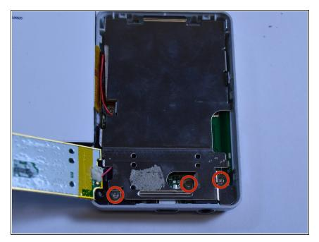
Use a Phillips Head screwdriver to unscrew the three 3/16 inch screws that were underneath the button input chip.
