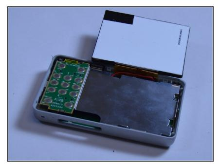
Flip the LCD screen off the midsection plate to gain access to the space around the input button chip.
