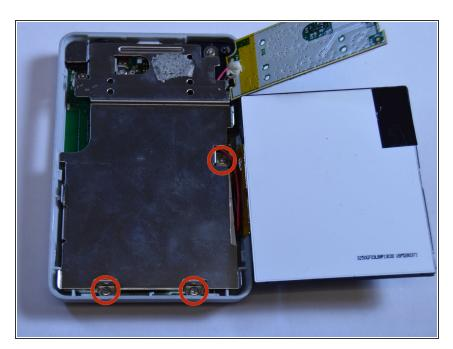
Use a Phillips Head screwdriver to unscrew the three 3/16 inch screws that were underneath the LCD screen.
