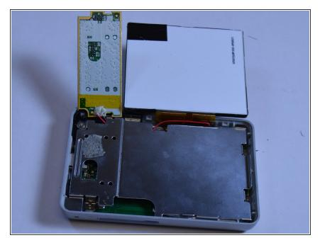
Lift open the LCD screen and button input chip to access the entire midsection plate.
