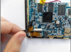
• Remove the black tape covering the cameras power cable.
