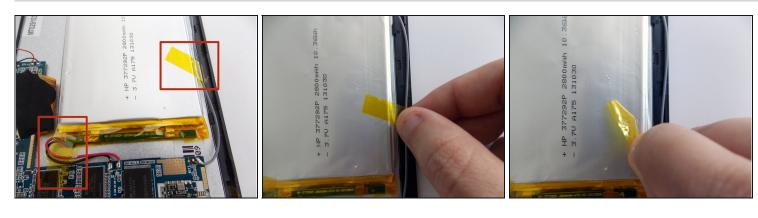
Remove the tape holding the battery in place.
