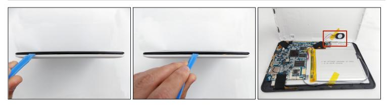
• With the plastic opening tool in the opening between the two sides of the case, slide the tool along the tablet's border to separate the two sides completely.
