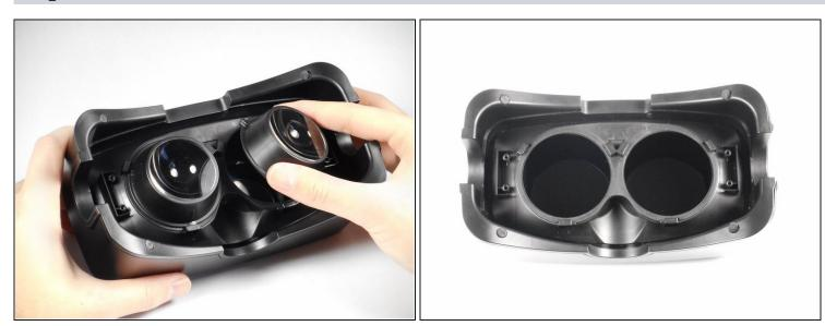
• With the Oculus facing up, twist the right lens clockwise and lift it out. Repeat for the left lens twisting counterclockwise instead.
