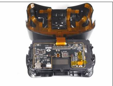
• Carefully separate the faceplate and the cover. Gently rest the cover plate on top of the faceplate as shown in the pictures.
