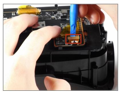
Lift the tape and gently pry up the video data ribbon cable using the plastic opening tool as shown.
