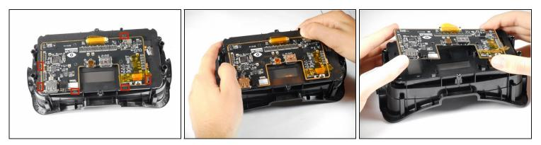
• Gently pry back the motherboard clips to release the motherboard. The motherboard should now lift free.
