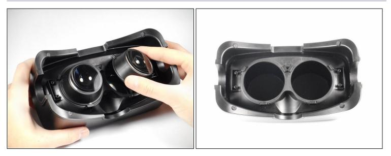
• With the Oculus facing up, twist the right lens clockwise and lift it out. Repeat for the left lens twisting counterclockwise instead.
