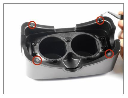
• Using <u>tweezers</u>, carefully lift the four rubber plugs as shown. They are a bit snug and you may need to jiggle them free with the tweezers.
