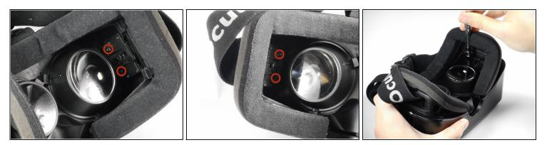
• Remove the four 3/8" Phillips #0 screws from the inner portion of the headset.
