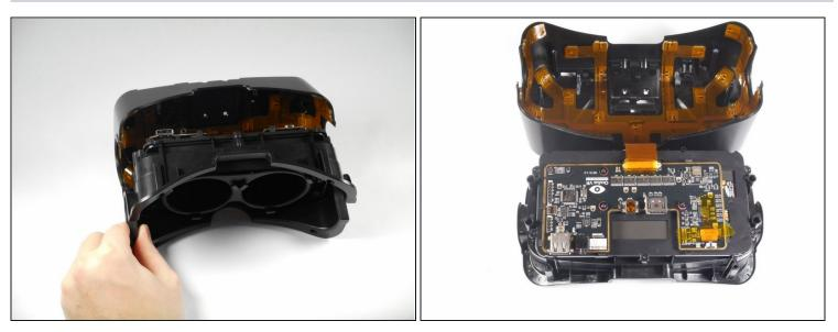
• Carefully separate the faceplate and the cover. Gently rest the cover plate on top of the faceplate as shown in the pictures.
