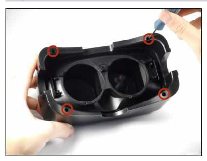
Remove the four 3/8" screws attaching the eyewear enclosure to the front casing.
