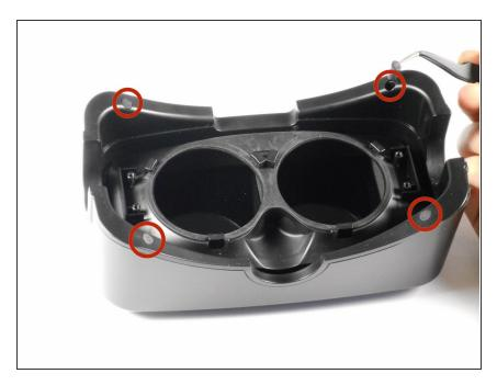
Using tweezers, carefully lift the four rubber plugs as shown. They are a bit snug and you may need to jiggle them free with the tweezers.
