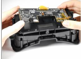
Gently pry back the motherboard clips to release the motherboard. The motherboard should now lift free.
