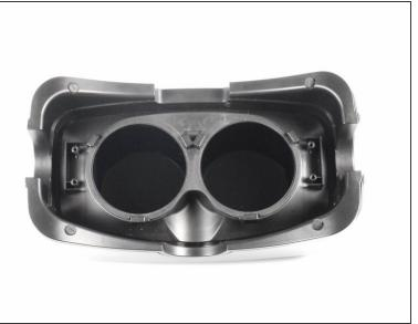
With the Oculus facing up, twist the right lens clockwise and lift it out. Repeat for the left lens twisting counterclockwise instead.
