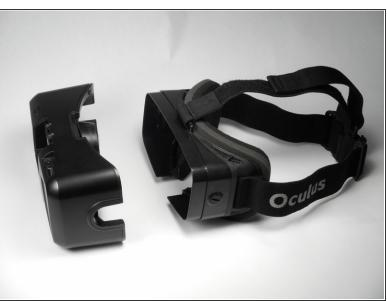
With the screws removed, gently pull the headband frame apart from the headset.
