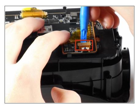
Lift the tape and gently pry up the video data ribbon cable using the plastic opening tool as shown.
