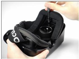
• Remove the four 3/8" Phillips #0 screws from the inner portion of the headset.
