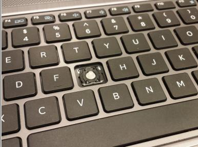
To clean underneath the keys, canned air works well.
