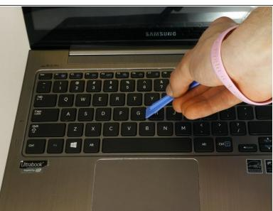
To take off the keys, simply use the plastic opening tool or a similar pointed object to take off the desired key(s).
