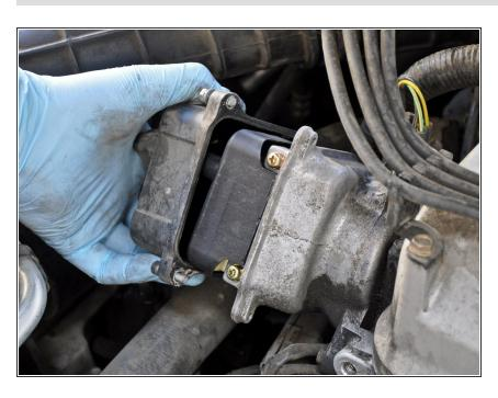
Pull the distributor cap away from the engine and set it aside.
