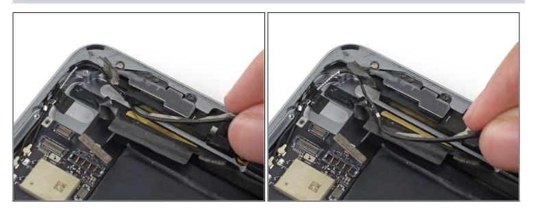
Pull the antenna cable out from under the corner of the right speaker.
