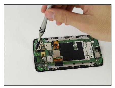
Remove the 2.3 mm T3 Torx screw on the top of the phone.
