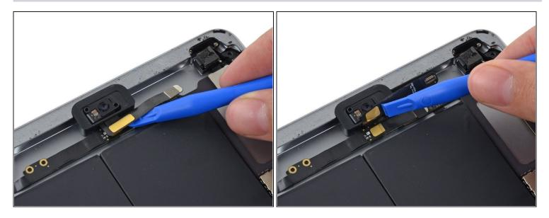
• Use a plastic opening tool to gently fold the front-facing camera cable upwards (roughly at a 90-degree angle), exposing the bottom side of it.
