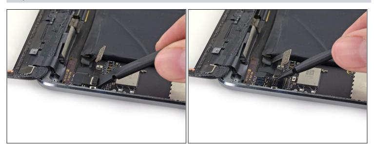
Use the flat end of a spudger to lift the digitizer cable connector straight up off of its socket.
