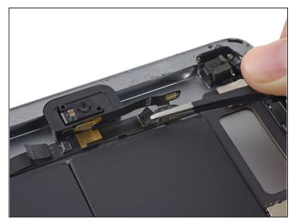
• Remove any tape covering the headphone jack cable connector.
