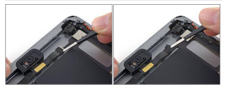
• Use a set of tweezers to remove any tape covering the front-facing camera cable clips.
