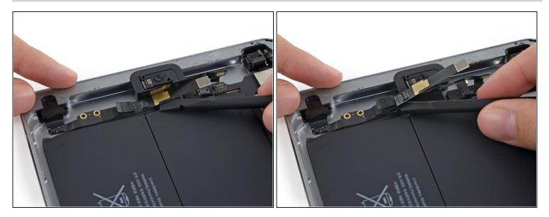
• Slide the flat end of a spudger beneath the length of the headphone jack cable, separating the adhesive securing the cable to the rear case.
